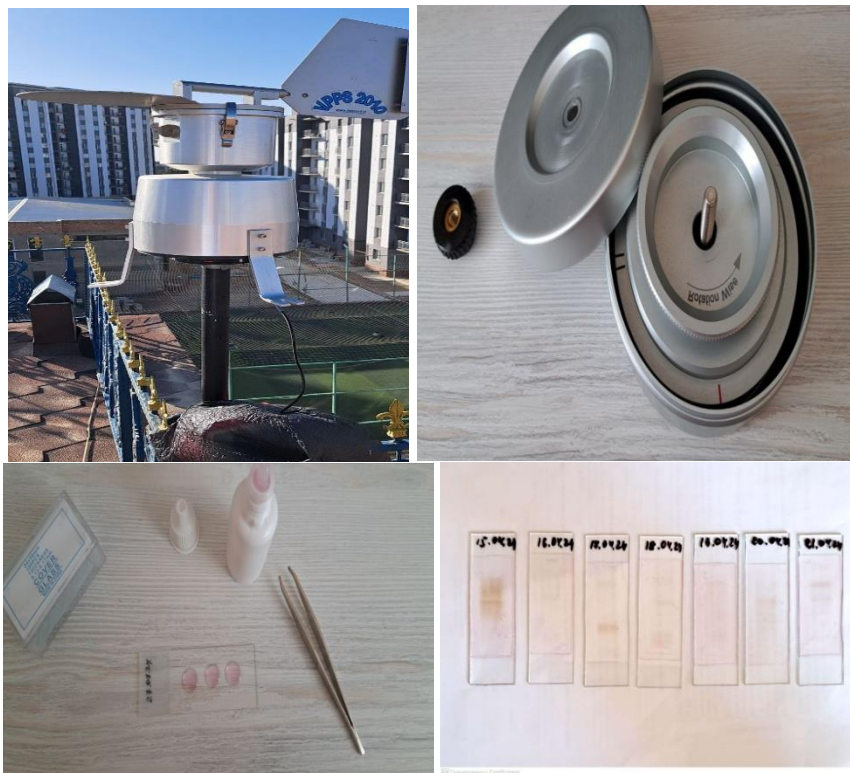
Figure – General view of the Lanzoni VPPS 2010 device and prepared microscopic slides
